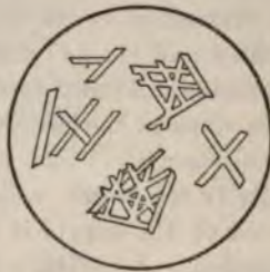
FIG. 5.—PLASTER CRYSTALS FORMING.
